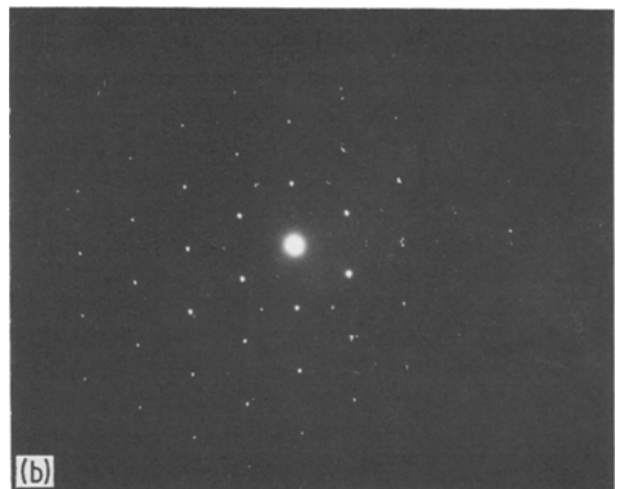
Figure 7 (a) Transmission electron microscopy and (b) electron diffraction images of hydrothermally obtained \text{BaFe}_{12}\text{O}_{19} .
